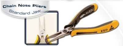
Features very fine tips, "eased" edges of the inner jaw to reduce the risk of damage to the workpiece during forming, and a long jaw for extended gripping power. Available with smooth or serrated jaws. Tip Dimensions: 1.2mm W x 1.4mm H (.050" x .060")
