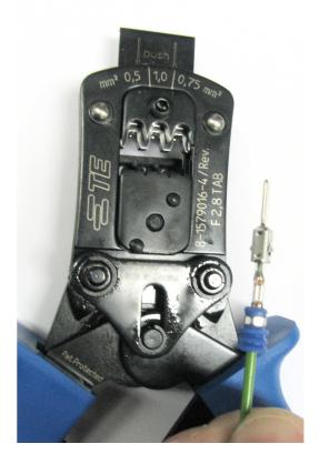
Picture 10: Checking the crimping contact
