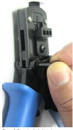
Picture 2: Removing the locking pins
