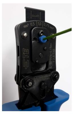
Picture 9: Closed crimp tool (crimping head)
