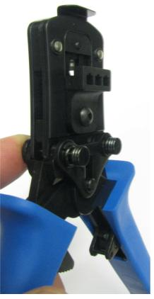
Pictrue 1: Pressing out the locking pins from the front
