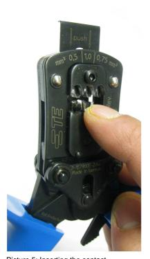
Picture 5: Inserting the contact
