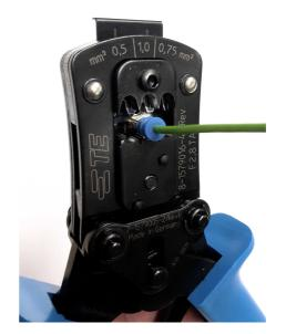
Picture 8: Insert the wire with the sealing ring
