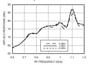
[1] Two-tone input power = +9 dBm each tone, 1 MHz spacing. [2] Referenced to RF Input power at 0 dBm
