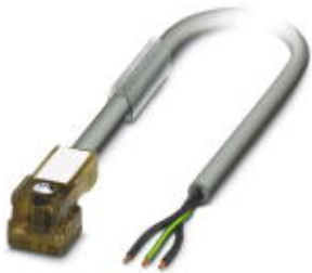
Sensor/Actuator cable, 3-position, PUR/PVC, Gray RAL 7001, free cable end, on Valve connector C (8 mm), with 1 LED, connected with Z diode, Cable length: 1.5 m
