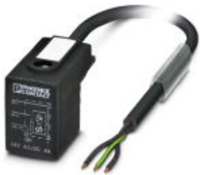
Sensor/Actuator cable, 3-position, PUR halogen-free, black-gray RAL 7021, free cable end, on Valve connector B (10 mm), with 1 LED, connected with Varistor, Cable length: 5 m
