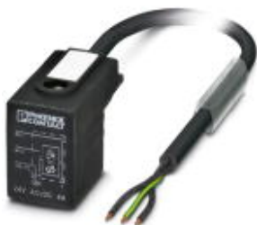
Sensor/Actuator cable, 3-position, PUR halogen-free, black-gray RAL 7021, free cable end, on Valve connector B (10 mm), with 1 LED, connected with Varistor, Cable length: 10 m
