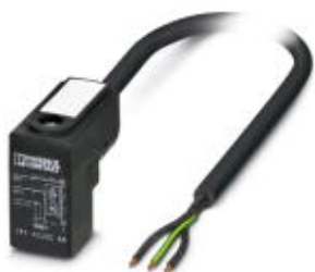
Sensor/Actuator cable, 3-position, PVC, Black RAL 9005, free cable end, on Valve connector C (8 mm), with 1 LED, connected with Z diode, Cable length: 2 m
