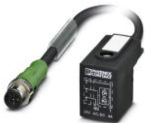
Sensor/Actuator cable, 3-position, PUR halogen-free, black-gray RAL 7021, Plug straight M12 SPEEDCON, A-coded, on Valve connector B (10 mm), with 1 LED, connected with Z diode, Cable length: 0.3 m
