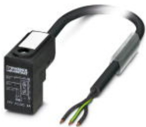
Sensor/Actuator cable, 3-position, PUR halogen-free, black-gray RAL 7021, free cable end, on Valve connector CI (9.4 mm), with 1 LED, connected with Varistor, Cable length: 10 m
