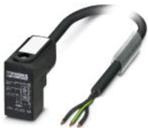
Sensor/Actuator cable, 3-position, PUR halogen-free, black-gray RAL 7021, free cable end, on Valve connector CI (9.4 mm), with 1 LED, connected with Z diode, Cable length: 1.5 m
