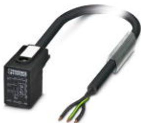
Sensor/Actuator cable, 3-position, PUR halogen-free, black-gray RAL 7021, free cable end, on Valve connector B (10 mm), with 1 LED, connected with Z diode, Cable length: 10 m
