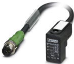
Sensor/Actuator cable, 3-position, PUR halogen-free, black-gray RAL 7021, Plug straight M12 SPEEDCON, A-coded, on Valve connector CI (9.4 mm), with 1 LED, connected with Z diode, Cable length: 3 m
