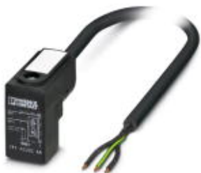
Sensor/Actuator cable, 3-position, PVC, Black RAL 9005, free cable end, on Valve connector C (8 mm), with 1 LED, connected with Z diode, Cable length: 5 m
