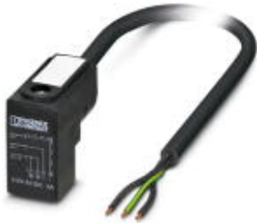
Sensor/Actuator cable, 3-position, PVC, Black RAL 9005, free cable end, on Valve connector CI (9.4 mm), Cable length: 2 m
