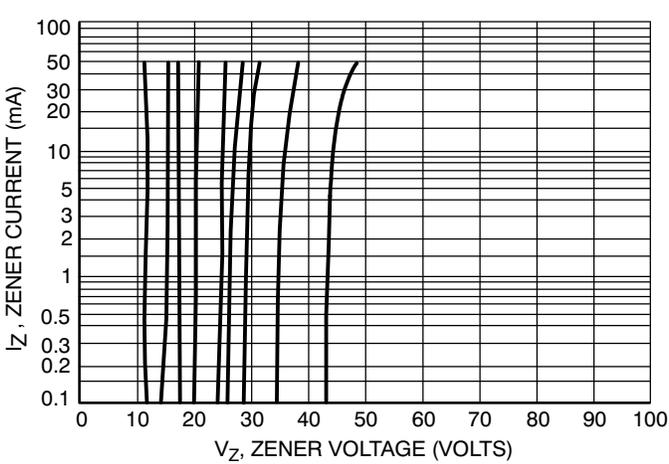
Figure 3.  $V_Z = 12$  thru 47 Volts
