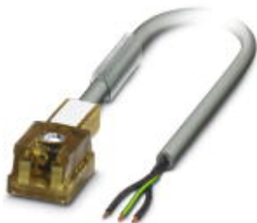
Sensor/Actuator cable, 3-position, PUR/PVC, Gray RAL 7001, free cable end, on Valve connector BI (11 mm), with 1 LED, connected with Z diode, Cable length: 5 m
