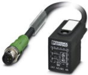
Sensor/Actuator cable, 3-position, PUR halogen-free, black-gray RAL 7021, Plug straight M12 SPEEDCON, A-coded, on Valve connector BI (11 mm), with 1 LED, connected with Z diode, Cable length: 1.5 m
