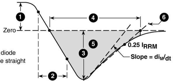
**Figure 2. Diode Reverse Recovery Waveform and Definitions**
