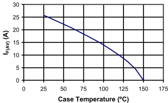
Figure 2. Maximum Average Forward Current vs. Case Temperature
