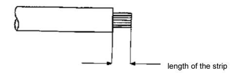
appropriate length: the length of wire barrel of used contact +0.5 $\sim$ 1.0mm
