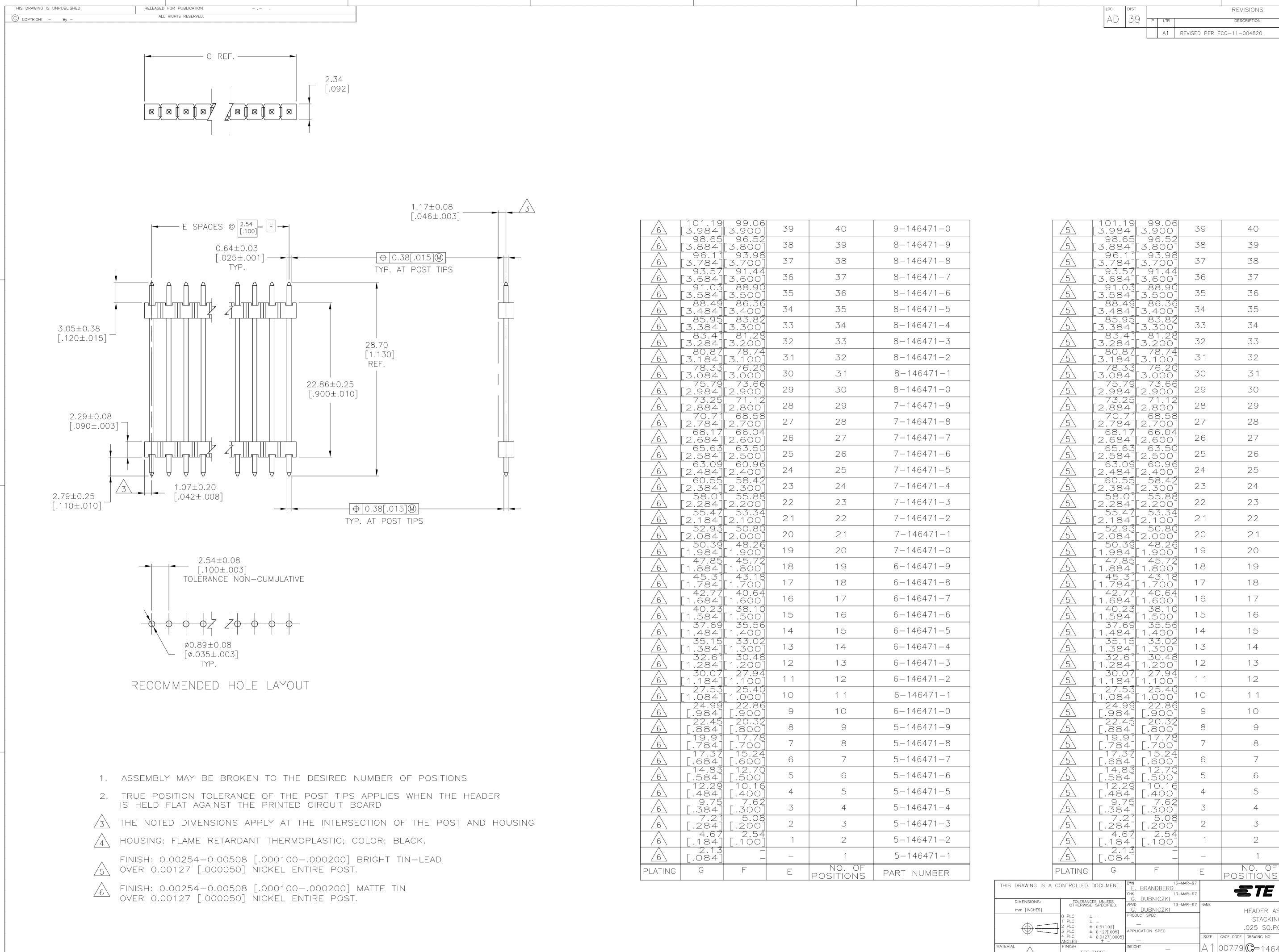
TE Connectivity HEADER ASSEMBLY, MOD II, STACKING, SINGLE ROW, .025 SQ.POST, UNSHROUDED SIZE CAGE CODE DRAWING NO 1 00779 **C-**146471 SEE TABLE SCALE 4:1 SHEET 1 OF REV A1 USTOMER DRAWING
