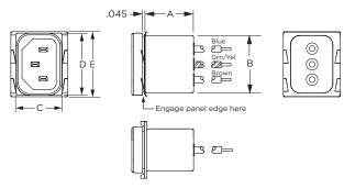
Typical Dimensions: Line Inlet (1): Wire Leads:
