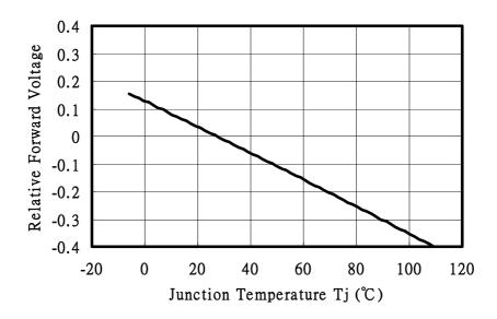
Note :  $\triangle V_F = V_F - V_F (25 \degree C) = f(Tj); I_F=2mA$
