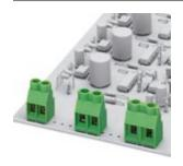
PCB terminal block, nominal current: 32 A, nom. voltage: 630 V, pitch: 9.52 mm, number of positions: 3, connection method: Screw connection with tension sleeve, mounting: Wave soldering, conductor/PCB connection direction: 0 °, color: black, The article can be aligned to create different nos. of positions!
