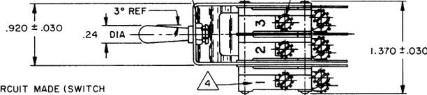
N.O. TO C CIRCUIT MADE (SWITCH NO. 4,5 AND 6) N.C. TO C CIRCUIT MADE (SWITCH NO. 1,2 AND 3) (MAINTAINED POSITION)
