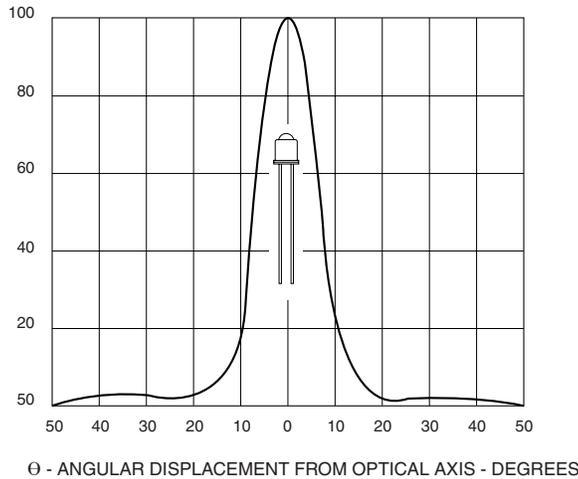
**Fig. 5 Typical Radiation Pattern**
