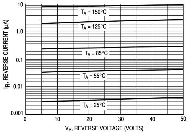
Figure 2. Leakage Current
