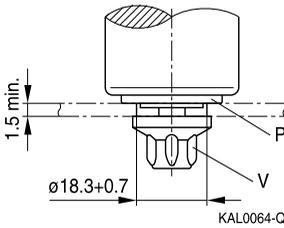
Insulated mounting with cap nut
