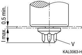
Non-insulated mounting with cap nut
