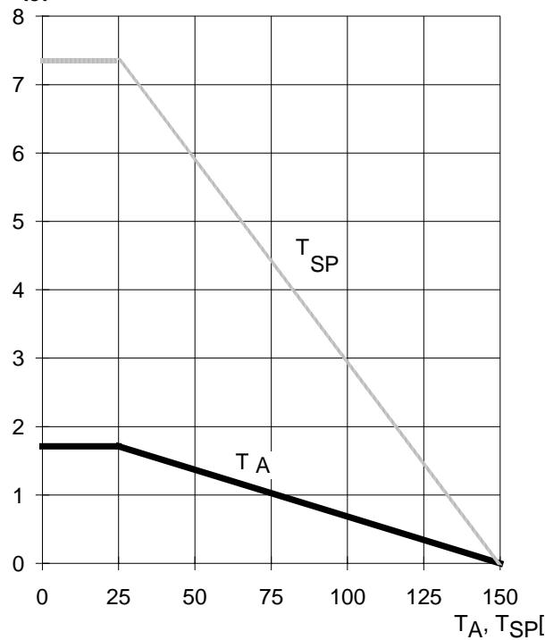
**Typ. on state resistance (V<sub>bb</sub>- pin to OUT pin)**
