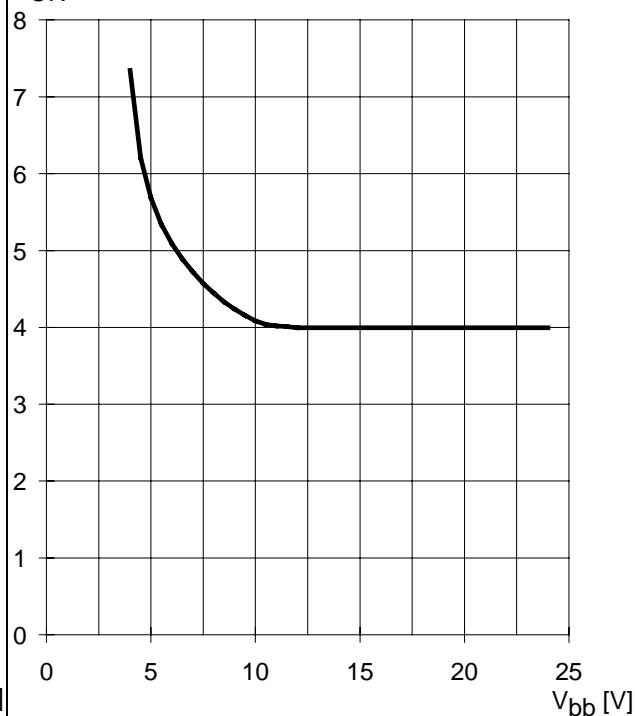
**On state resistance (V<sub>bb</sub>- pin to OUT pin)**
