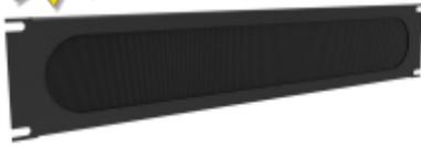
The Brushed Rack Panel (BRP) reduces unwanted airflow inside a rack cabinet while allowing cables to pass through to the reverse side. The BRP includes a cable management tray that reduces cable fatigue and an area to secure cables.
