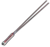
120 Series, standard glass probe, 2,000 Ohm resistance, ±20.0% tolerance, 25/85 BETA = 3518
