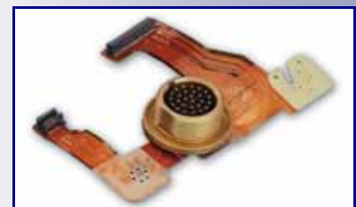
Flex Termination with MIL-C-26482 Special Connector
