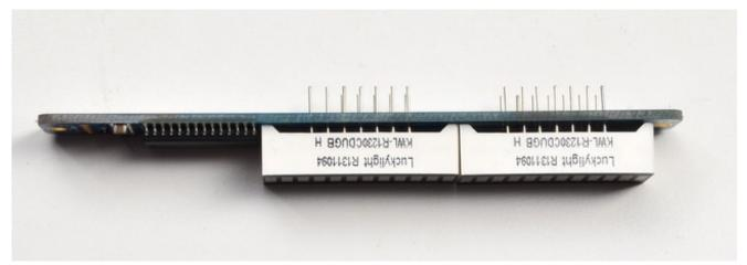
To keep the two bargraphs lined up nicely, you can use a little masking or scotch tape on the bargraph modules, tape them so they are in a straight line. There is a little play during soldering so if you don't do this the two modules may not be in a perfect line.
