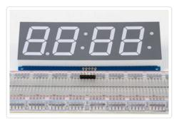
Cut the header strip to length if necessary and insert LONG pins down into the breadboard.
