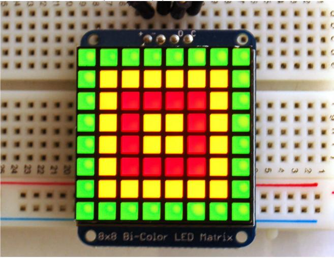
Pay close attention to the instructions for positioning the matrix. It must be oriented correctly to work and is almost impossible to remove it once it has been soldered to the backpack!
