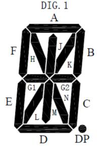
the 16 bit digit you pass in for raw image has this mapping:
