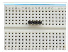
Break off a piece of male header, 4 pins long. Plug the **long ends** into a solderless breadboard.
