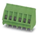
PCB terminal block, Nominal current: 24 A, Nom. voltage: 400 V, Pitch: 5.08 mm, Number of positions: 3, Connection method: Screw connection, Mounting: Soldering, Conductor/PCB connection direction: 35 °, Color: green, The article can be aligned to create different nos. of positions!
