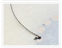
Dab a little Fray Check or clear nail polish on the knot while holding it tight. This will prevent the knot from coming undone and creating unwanted shorts in your circuit. Trim the tail very close to the knot.
