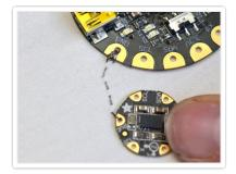
Stitch a path over to the gnd pad on the Flora accelerometer. When you get there, stitch a few times around the sensor's gnd pad.
