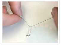
Stitch a few times around the GND pad and end on the back side of the fabric. Tie the tail and the working thread into a square knot, tight against the fabric.
