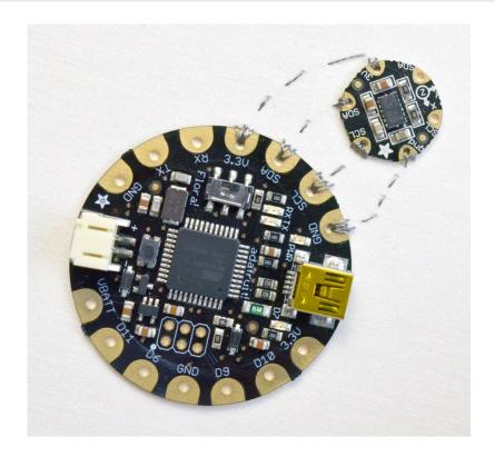
Repeat this process to make the other three required connections to the accelerometer - 3.3v, SCL, and SDA. This is the i2c bus on the Flora, and you can chain more sensors (http://adafru.it/1246) (or LED matrix backpacks (http://adafru.it/aQg)) to this first one by connecting to the as-of-now unconnected SDA and SCL pins. i2c is great for this application because you can connect many devices to each other without using up all the pins on the Flora.
