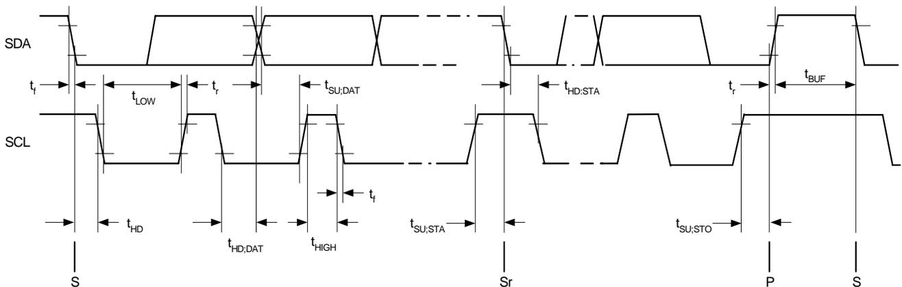
Figure 7. I<sup>2</sup>C Timing Diagram
