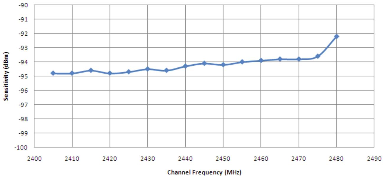
Figure 3. Typical RX Sensitivity vs. Channel Frequency @ 25°C
