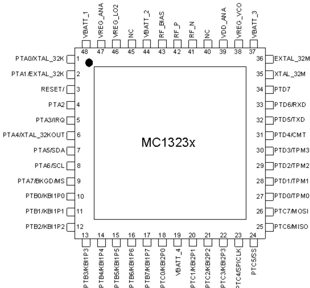
Figure 2. MC1323x Pinout
