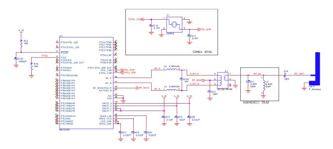
Figure 8. MC13233x Basic Applications Circuit
