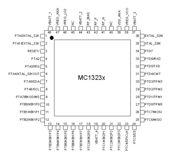
Figure 2. MC1323x Pinout
