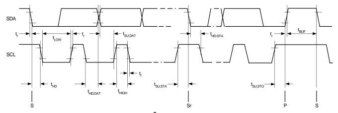
Figure 7. I<sup>2</sup>C Timing Diagram
