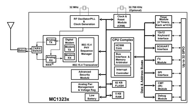
Figure 1. MC1323x Simplified Block Diagram
