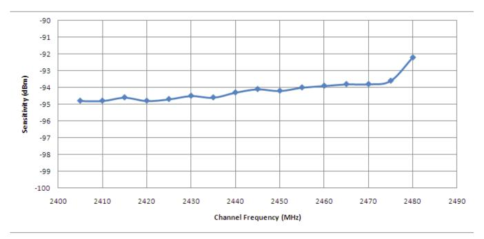
Figure 3. Typical RX Sensitivity vs. Channel Frequency @ 25°C
