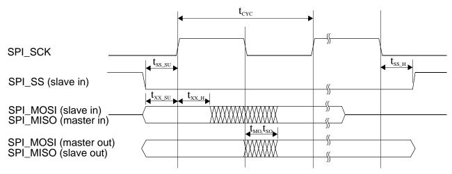
Figure 6. SPI Timing Diagram
