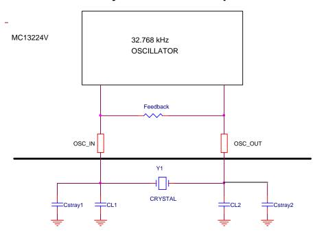
Figure 5. 32.768 kHz Oscillator Mode
