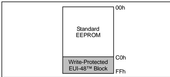
The 6-byte EUI-48™ node address value is stored in array locations 0xFA through 0xFF, as shown in Figure 3-2. The first 3 bytes are the Organizationally Unique Identifier (OUI) assigned to Microchip by the IEEE Registration Authority. The remaining 3 bytes are the Extension Identifier, and are generated by Microchip to ensure a globally-unique, 48-bit value.
