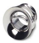
Pressure screws, with flared cable guard, clamping area 8 mm  $\dots$  13.5 mm, for housing with Pg13.5 support
