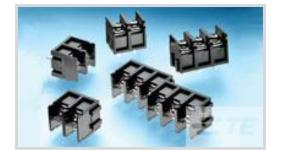
Barrier Strip Style: Dual Barrier Bottom Termination Style: Printed Circuit Pin Current Rating: 15 A Number of Positions: 16 Centerline (Pitch): 8.26 mm [.325 in ]
