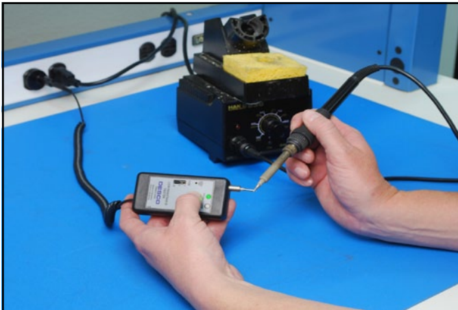
Figure 4. Testing soldering iron with 19245 tester.
