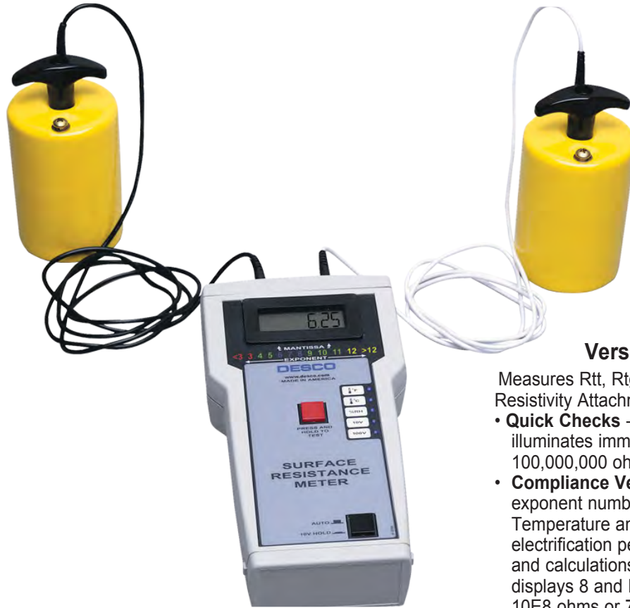
Figure 1. Desco 19780 Surface Resistance Test Kit
