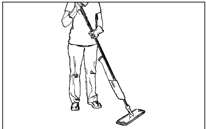
Figure 6. Applying floor finish with Flat Mop (optional).
