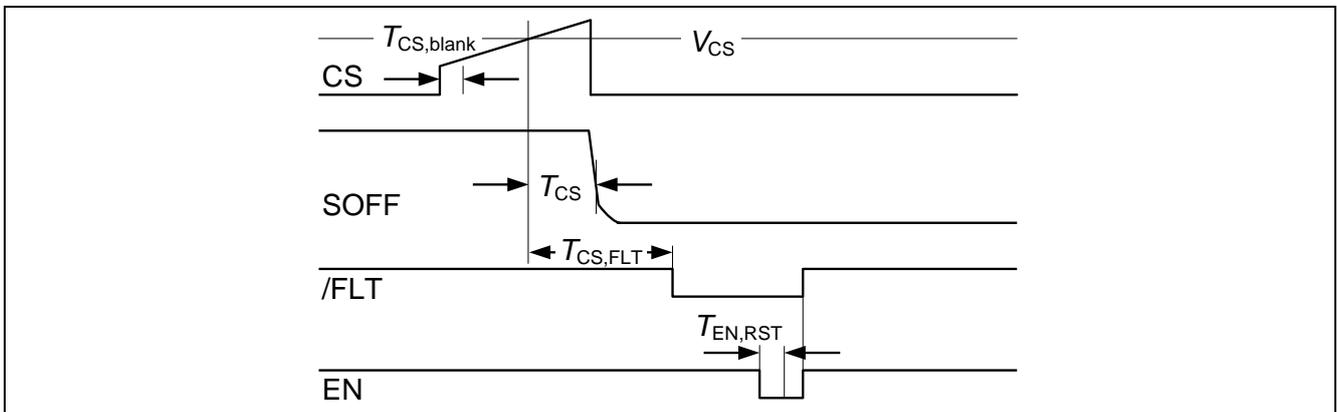
Figure 13 Timing of CS events incl. terminals SOFF, /FLT and EN
