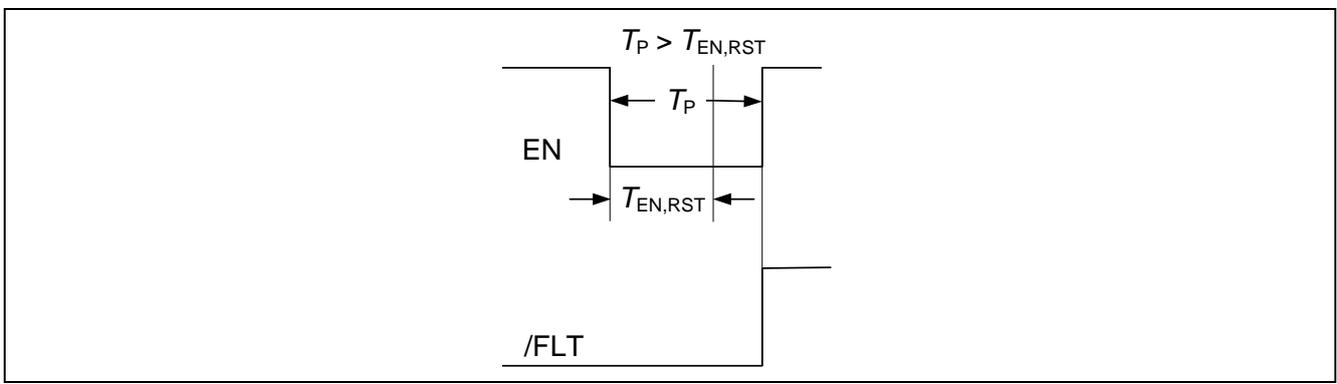
Figure 12 Timing for fault reset at terminal EN
