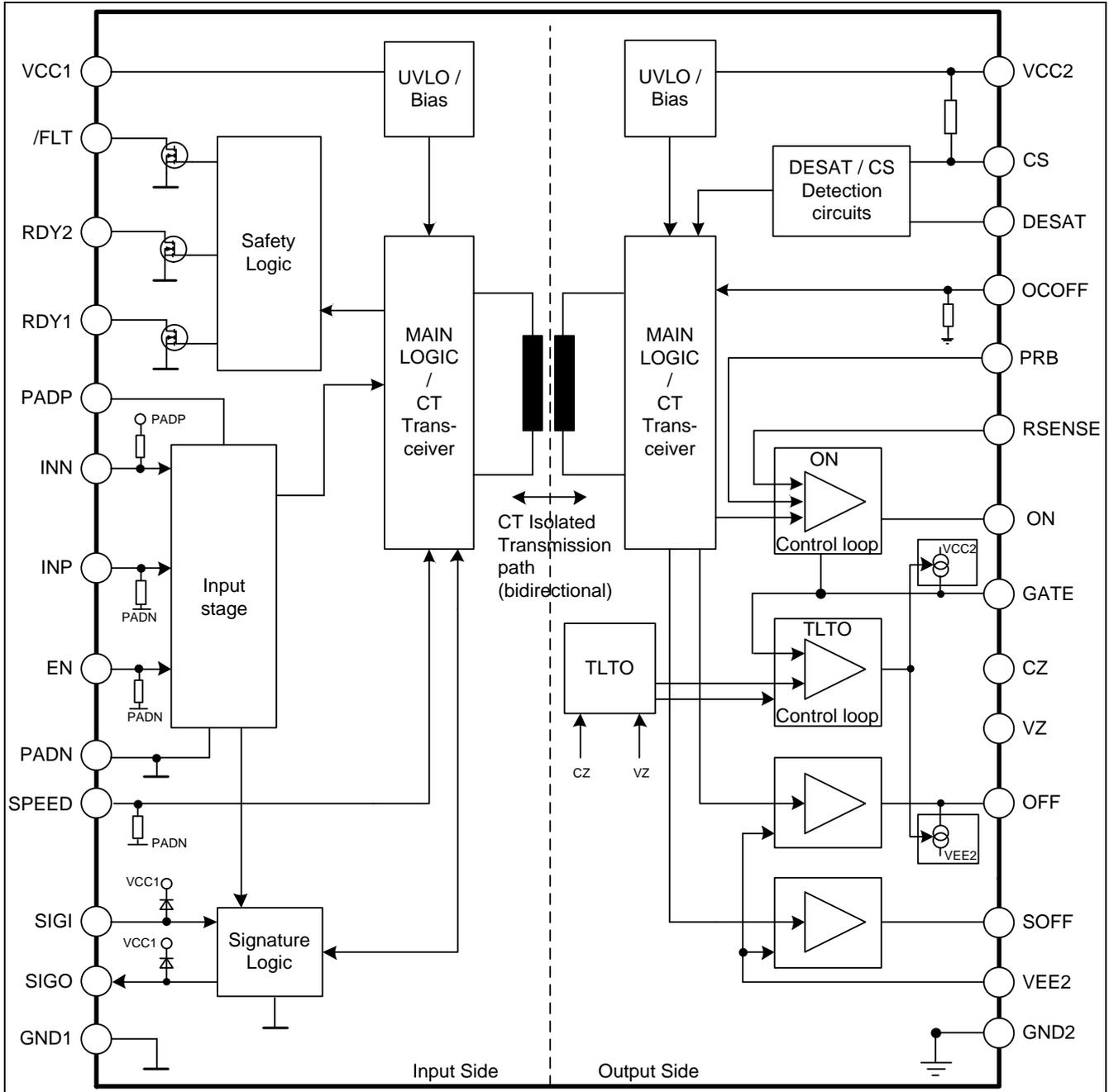
Figure 1 Block diagram for the 1EDS-SRC family
