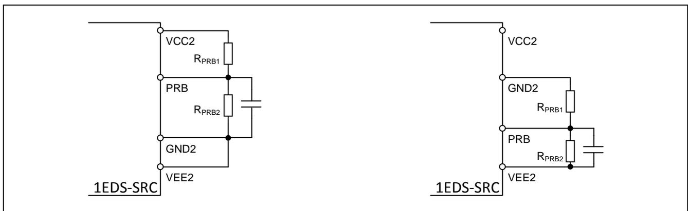
**Figure 5 External circuit for setting of preboost current (left: unipolar supply; right: bipolar supply)**
