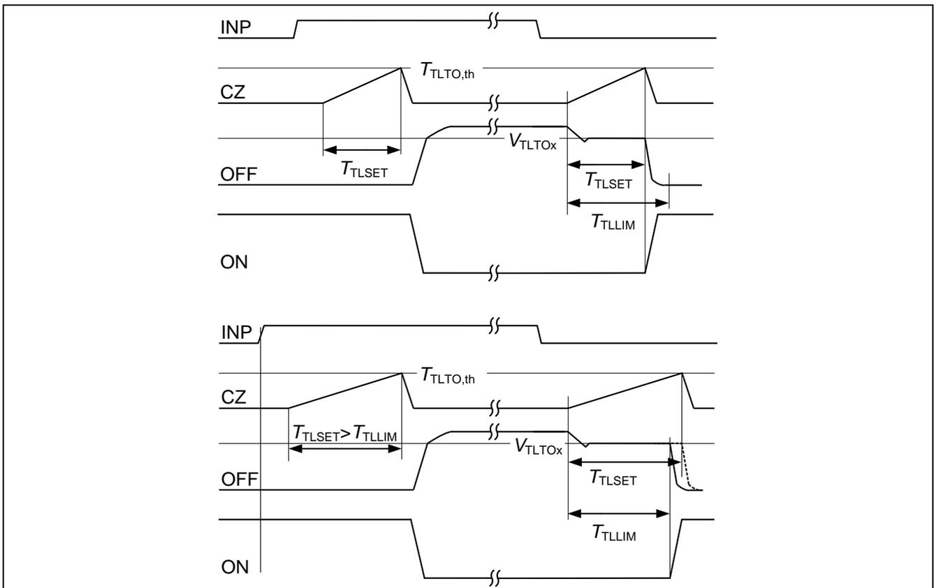
Figure 15 Timing for two-level turn-off incl. terminals CZ and OFF
