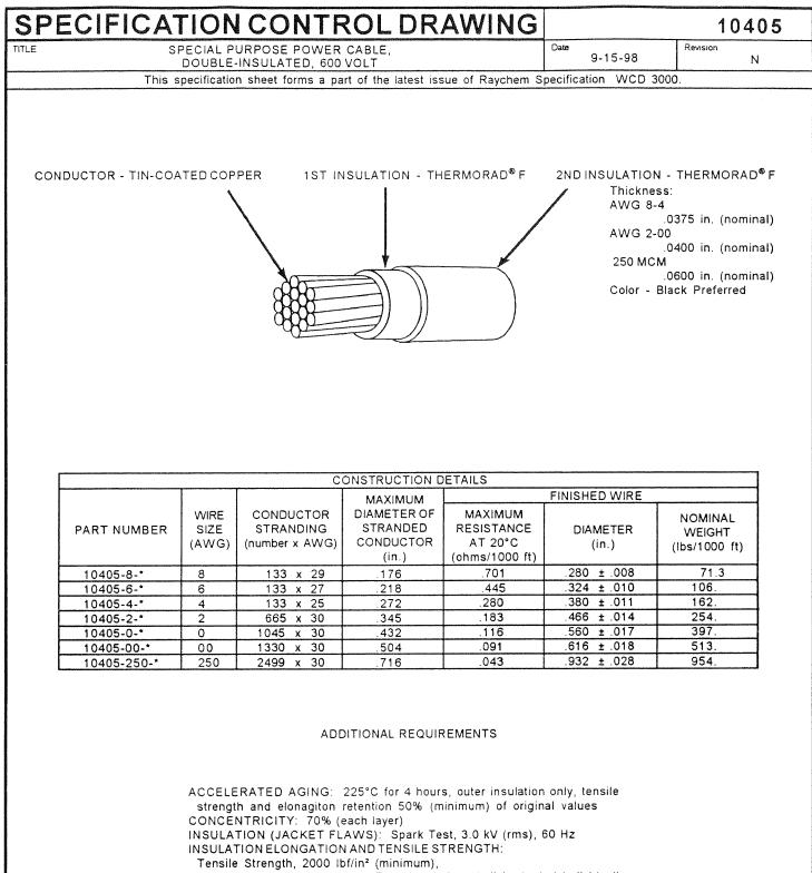
Elongation, 300% (minimum), Each insulation shall be tested individually for Tensile Strength and Elongation.
