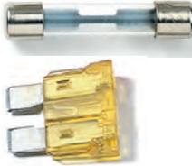
If an overcurrent causes the current in a circuit to rise above a specific level — often the circuit’s rating — the heat produced will melt the fuse’s element, causing the fuse to “blow.” This opens the circuit and immediately stops the flow of current. Fuses are designed to blow at temperatures far below those that would cause damage or hazards.
