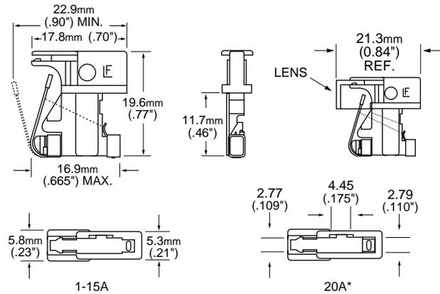
\*20A Fuseholder must be used. Fuse is keyed to prevent insertion in lower rated holders. 20A Fuseholder is designed to accept all ratings up to 20 amperes.
