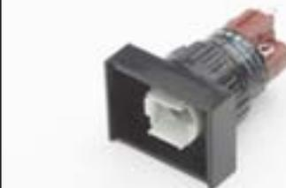
Illuminated pushbutton actuator, snap-action, raised, rectangular, black plastic, 16mm mounting, solder terminals, gold over silver contacts
