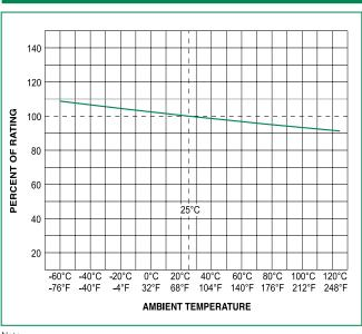
1) Rerating depicted in this curve is in addition to the standard rerating of 25% for continuous operation.
