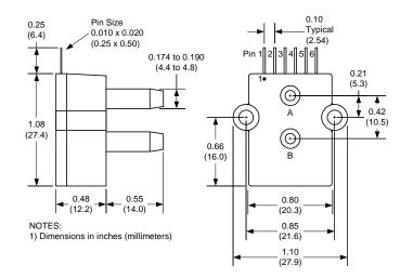
pin 1: N/C pin 2: +V supply pin 3: +Voutput pin 4: -Vsupply
