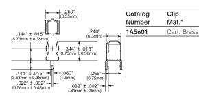
1A5602 Series For 5mm Diameter Fuses (0 to 7 Amps)
